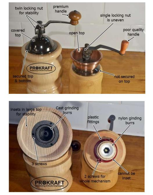
The primary reason the Prokraft grinder is different from most is that the entire grinder mechanism is inset in the lid of the grinder. This means a larger blank is required but it also means that the finished piece is heavier and much more stable in use.
